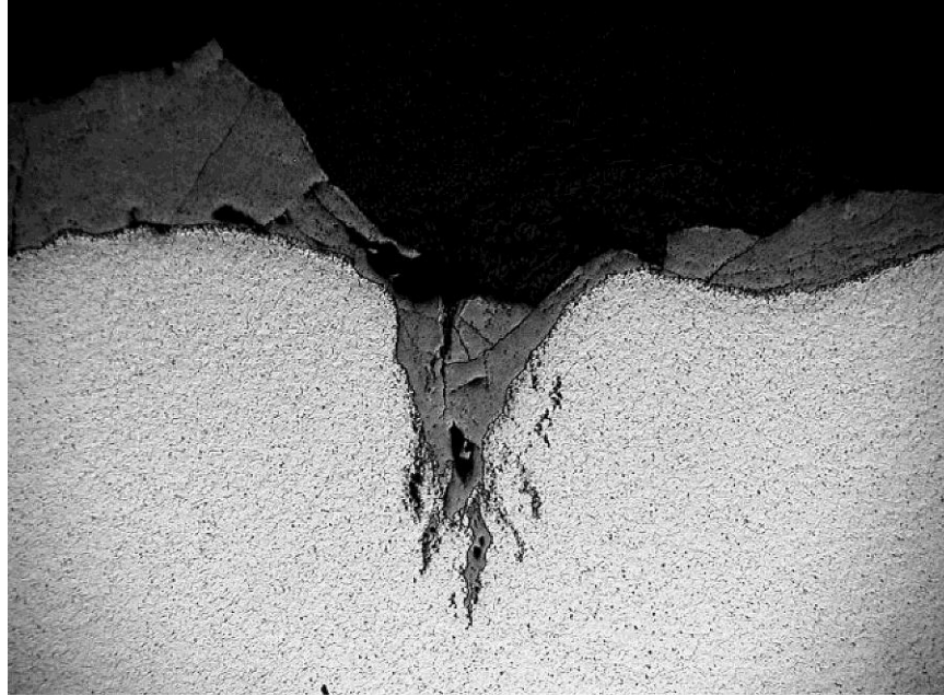
Figure 2. Tube wastage and creep damage, reheater T22 tube, OD. 80x.
