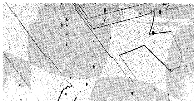
Fig. 1. Normal austenitic, stainless-steel microstructure is equiaxed grains. 500x, etched.
