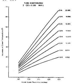
For the cooler tubes a small increase of 25° - 35°F is of no significance. How-ever, for the hottest ones such an increase can be devastating. Thus, the suggested metallurgical evaluation should include a characterization of the internal scale thickness. By keeping good records of failures, by cataloguing the kinds; high temperature creep, ash corrosion, weld related, the amount of tube wastage, spacer and attachment, by mapping the location, the overall metallurgical condition is more easily
