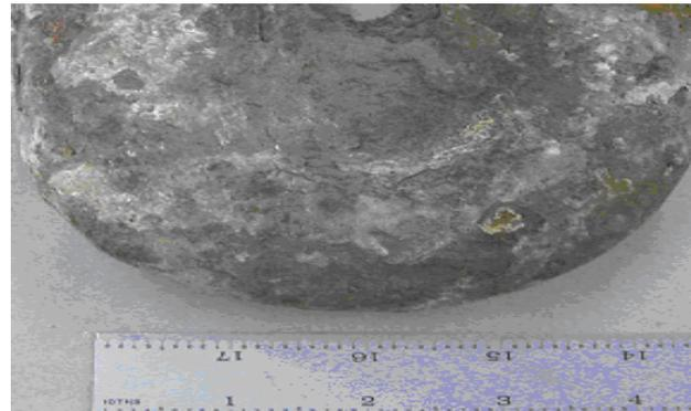
Corrosion on the higher-temperature regions of the superheater tubes depends on the fuel and impurities in the fuel. The culprits that lead to rapid corrosion wastage for oil-fired boilers are ash constituents of vanadium, sodium, and sulfur. Impurities and the compounds they form cause corrosion and are exacerbated by the addition of chlorine. Seawater in oil that is transported in ocean-going vessels will find a way to the ash deposits after combustion. The most serious form of fire-side
