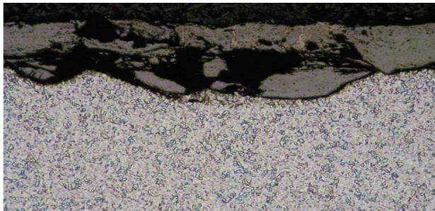
removed, the surface of the steel will have an “alligator hide” appearance formed as shallow grooves have penetrated the steel in a cross hatched pattern.
