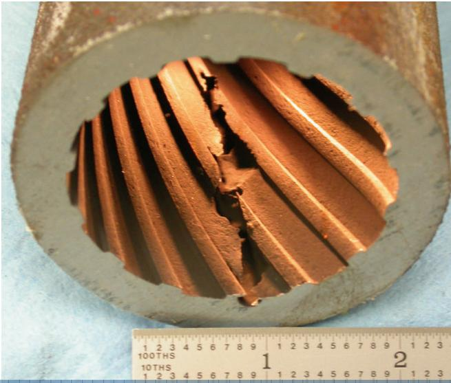
Caustic attack in a furnace division wall tube at a burner elevation
