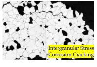
stresses may be either or both; for example, the hoop stress in a tube from the internal steam-water pressure for a residual stress from cold work. The most common occurrence develops at room temperature where obviously water is a liquid and present. It can occur at higher pressures but again water needs to be liquid for the damage to occur. Removing either the stress or the chlorides will prevent cracking.
